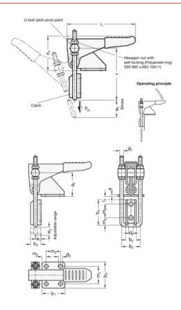
\* = With standart latch b2 = 44 d1 = M6 h1 = 54 l1 = 106 Newton = 3200 r = 54\* w2 = 21\*
